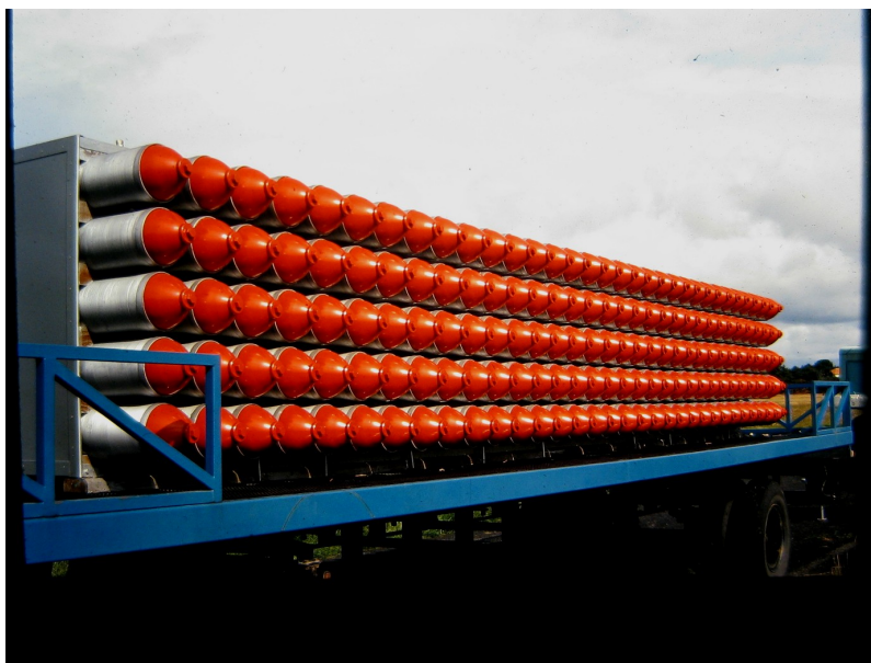
Storing Hydrogen: Inflating a high-altitude balloon takes 160 cylinders of hydrogen. They need a truck to carry them around.
